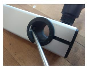
The plastic sleeves that are fitted into each end of the arm do need to be removed, as these will be replaced. Loosen or remove the tightening handle first. A pick or screwdriver helps, and these will be discarded.
