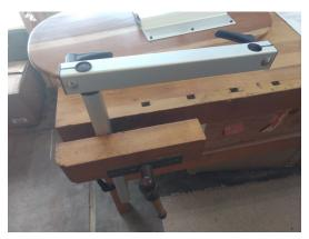
The root cause is the plastic bearings at each end of the arm, shown here. Each bearing assembly has an inner cylinder and an outer ring.
