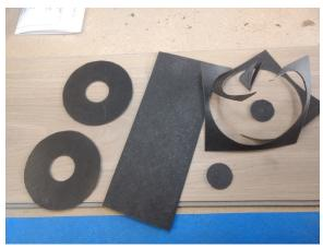
I cut some large "washers" from a heavy plastic report cover sleeve. I used only one of them, between the arm and the table mount. This serves as a low(er) friction surface as the table rotates.
