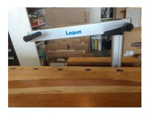
Here's the basic problem. Once the plastic bearings wear, the arm supporting the table (table not shown here) begins to sag. The table will always tilt.
