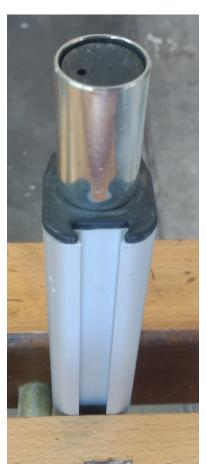
Slip the new metal bearing sleeve over the plastic post. Do the same on the table mount. The next step is to secure this in place, since there is just a bit of slop.
