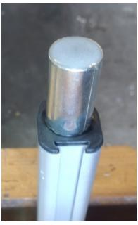
This is the key step. While holding the sleeve up in a half-installed position, mix up some epoxy and pour just a bit onto the post. Work the sleeve down over the post, making sure that the epoxy fills in the empty space around the sleeve. Once the sleeve is all the way down, add enough epoxy to finish the end, covering the plastic. Clean up any spillage.
