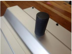
A similar inner bearing is integrated into the table mount. Do not remove this, either.
