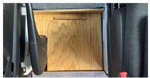
And here is the platform with no carpet, showing the cutout around the brake handle and the positioning bar that is fixed to the base.
