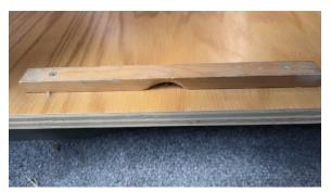
The locating block for the console box is screwed into the platform. The finger notch allows for easy removal to lift the platform floor up and forward.
