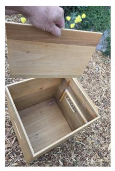
Here the panel is completely removed. The vertical support bars are quarter-rounded on the side facing the box top so as not to interfere with the top as it is dropped in.
