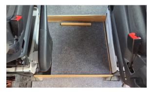
The first (and most tedious) step in construction is to build a level platform on which to rest the console box. Here the box is removed, showing the platform with a bit of carpet on it.
