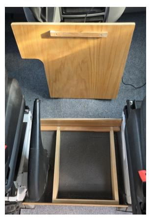
Here the top of the platform is removed by lifting the front edge and sliding the panel forward.
