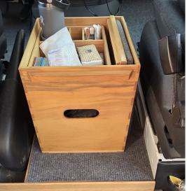
This console box was constructed in 2021 for our 2017 Sprinter camper. The sides are poplar (I think) of 5/16" thickness, and the top and bottom are 3/4" thick. The tray insert is from oak, also 5/16" thick.
