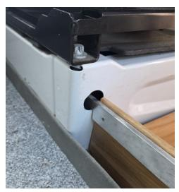
The crossbar is notched at each end to fit into the holes in the Sprinter's seat pedestal. This is the right side. The crossbar is positioned between the two holes, then the platform is screwed to it, securing the system in place.
